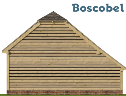
Catslide roof to rear
